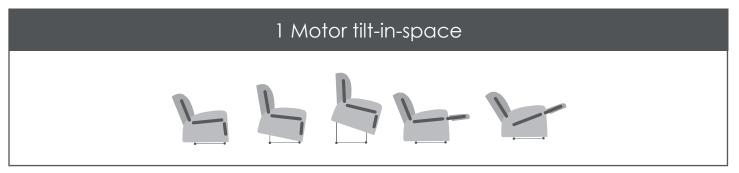
Tilt-in-space holds the user in a fixed position when in recline with the angle of the hip and the back remaining constant. This action is ideal for clients with limited torso control.
