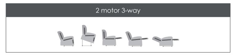
The back and footboard operate independently of each other with the benefit of being able to achieve optimum comfort in a seated or reclined position. The 2 motor mechanism also allows the back to recline independently at any point in the recline cycle.
